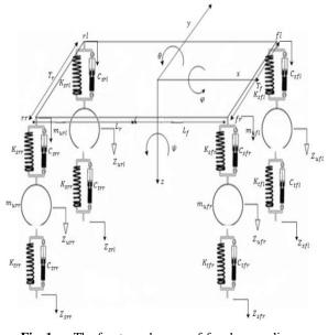
Fig. 1 The fourteen-degrees-of-freedom nonlinear dynamic model [15].
