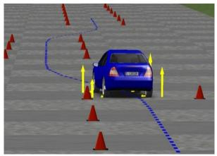
Fig. 3 The scheme of double lane change maneuver.
