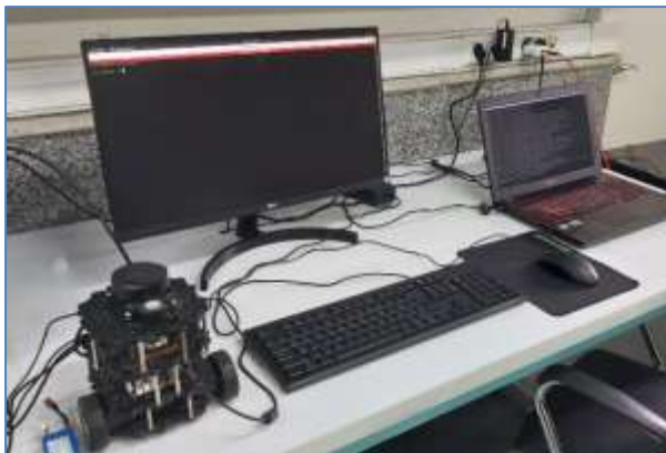
Fig. 9 The robot used for experimental tests (turtlebot3 burger), and the remote laptop used to control the robot.
