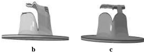
**Fig. 4** Comparison of the blank at the moment of failure: (a): Experimental test, (b): Based on GTN damage model, and (c): Based on Porous metal plasticity model
