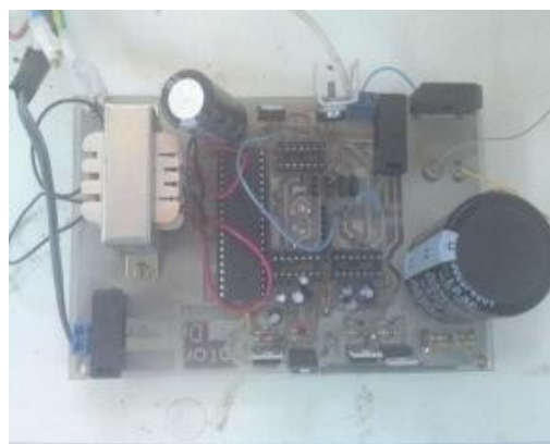
Fig. 19. The implemented inverter
