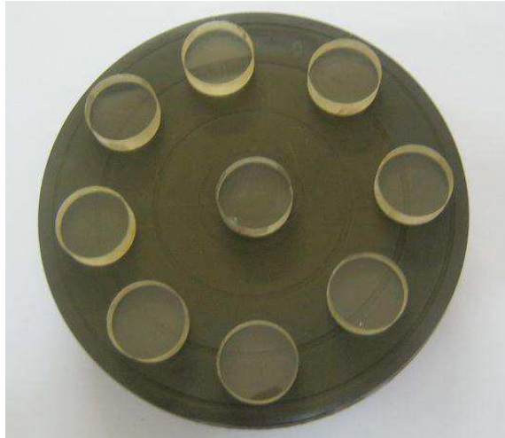
Figure2. Specimens are glued and prepared for milling with D91 diamond cup grinding tool
