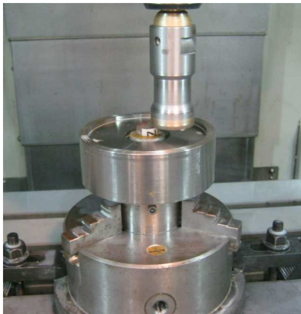
Figure3. Grinding test in brittle mode with D64 cup grinding tool
