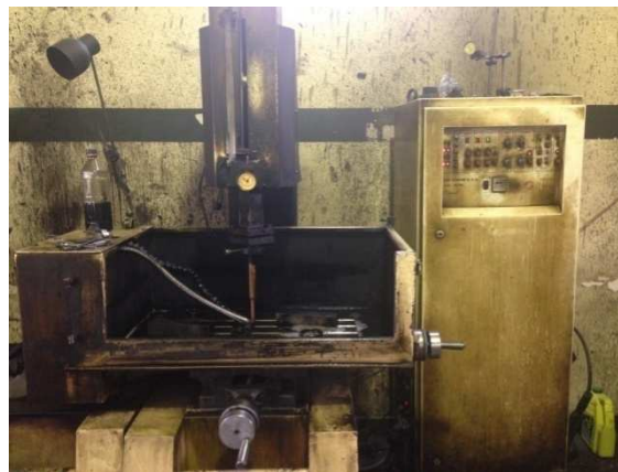
Figure 2. Spark machine model 50A-501
