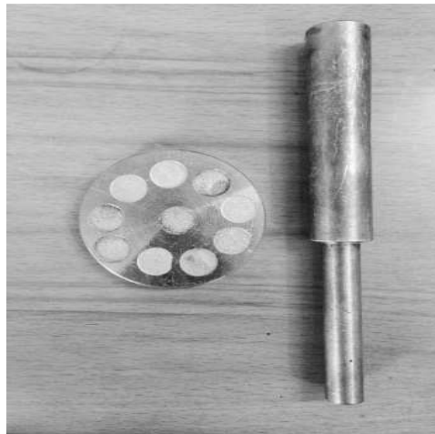
Figure 1. Sample and electrode utilized in EDM
