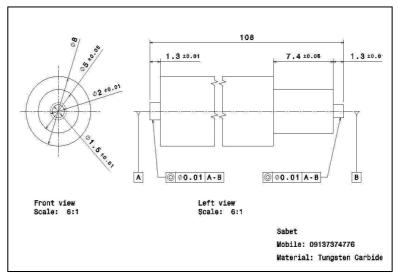
Figure2. Schematic view of manufactured tool
