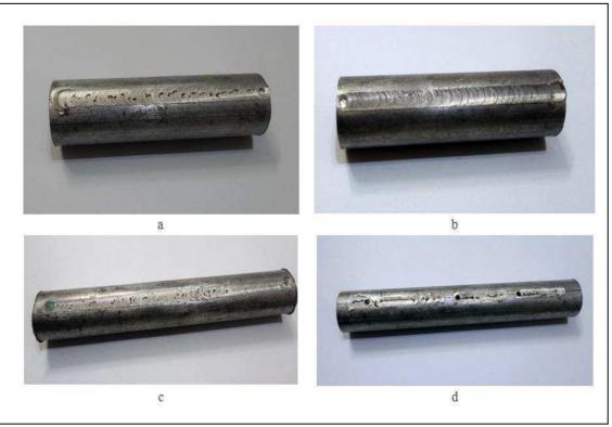
Figure4. Welded piece using frictional stir welding tube process: a) Rotational speed of 2000 rpm and welding speed of 12mm/min b) Rotational speed of 2500 rpm and welding speed of 8 mm/min c) Rotational speed of 2000 rpm and welding speed of 4 mm/min d) Rotational speed of 1600 rpm and welding speed of 8 mm/min
