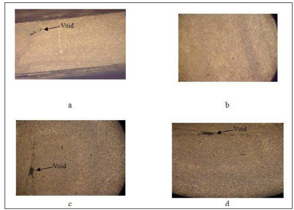
Figure 5. The macroscopic view of welded cross section in various welding parameters: a) Rotational speed of 2000 rpm and welding speed of 12mm/min b) Rotational speed of 2500 rpm and welding speed of 8 mm/min
