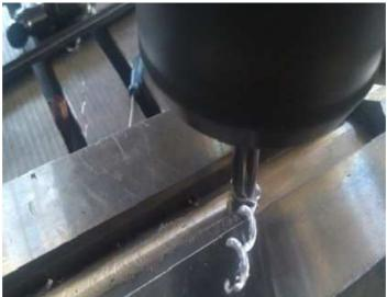
Figure3. Implementation of frictional stir welding process
