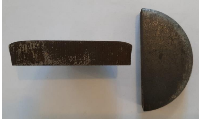
Figure 13. Cutting the blank produced by the wire electric discharge process and the cut cross-section of the blank
