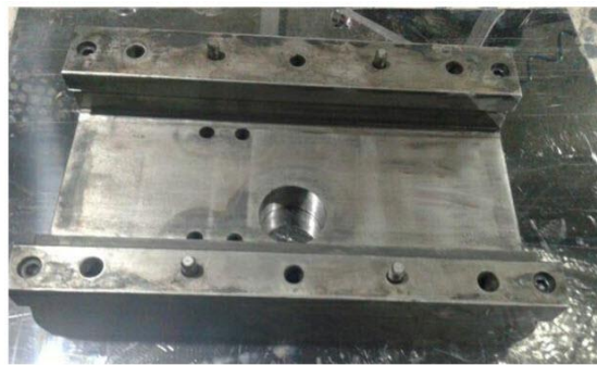
Figure 10. The feeding channel is mounted on the matrix and the lower shoe
