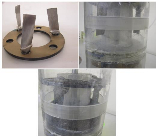
Figure 16. Blade and its setting condition in MAF machine with abrasive powder
