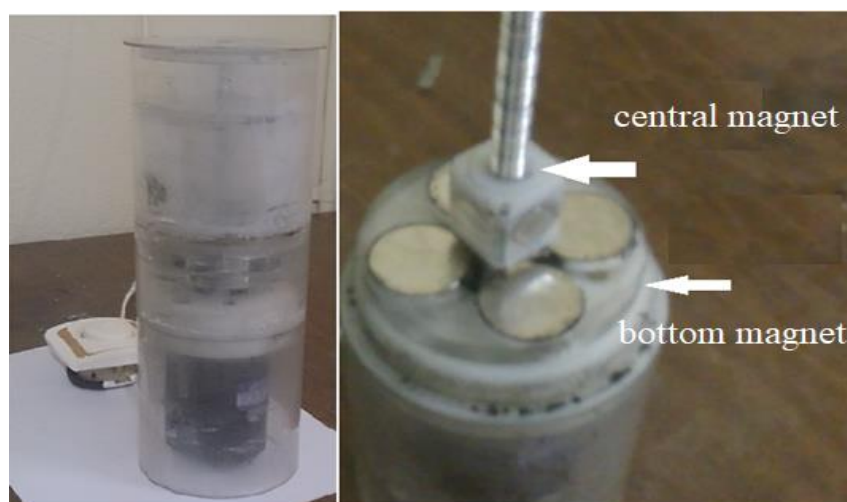
Figure 5. Location and setting condition of magnetic poles (16×Ø20mm) in plexiglass fixture
