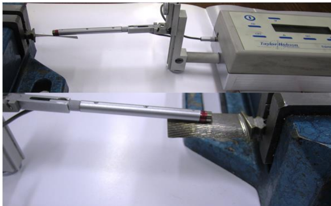
Figure 15. Measurement procedure of surface roughness of compressor blade
