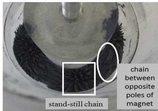
Figure 20. The development of chain and stand-still chain between opposite poles of the magnet
