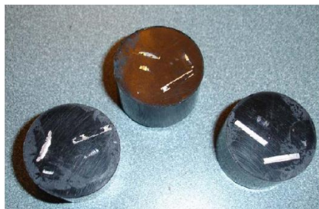
Figure 7. Schematic of several samples prepared for micro-hardness and microstructure testing
