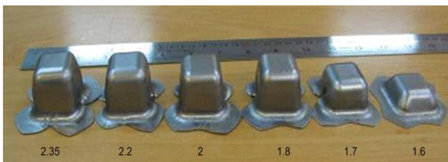
Figure 11. Perfect Parts in various drawing ratios
