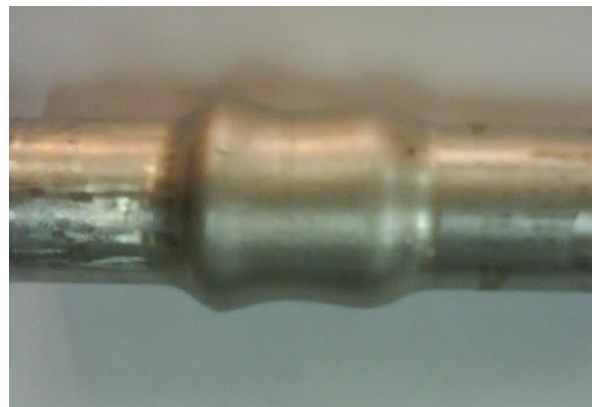
Figure 10. (a) Axial feeding curves (b) wrinkled part
