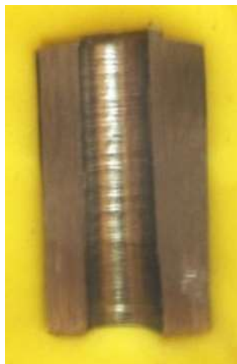
Figure2. Half of a samples which is cut and polished and ready for measurement.
