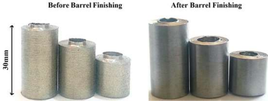
Figure12. Samples before and after 3 hours deburring with aluminum oxide as the abrasive media
