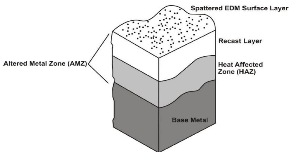
Figure1. Surface layers after EDM [2]
