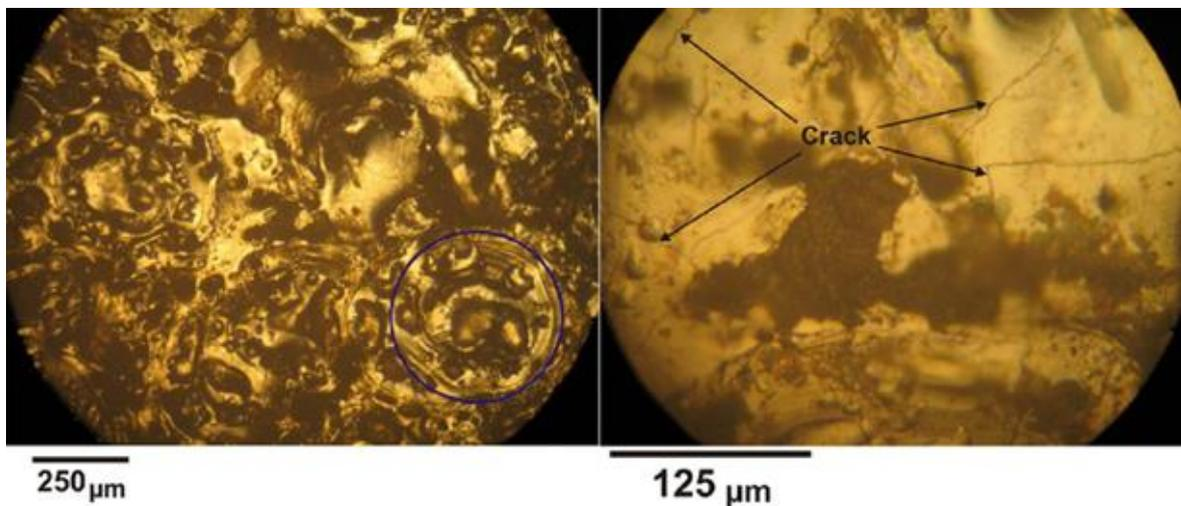
Figure9. Machining effect on samples with parameters set as, on-time = 800μs, off-time = 50μs, current (I) =5 A and voltage (V) =40 V, Right: observation of micro cracks, Left: circle surrounding the spark erosion zone
