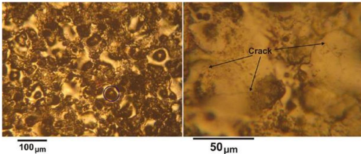
Figure8. Machining effect on samples with parameters set as, on-time = 50μs, off-time= 50μs, current (I) =1 A and voltage (V) =40 V, Right: observation of micro cracks, Left: circle surrounding a spark erosion zone
