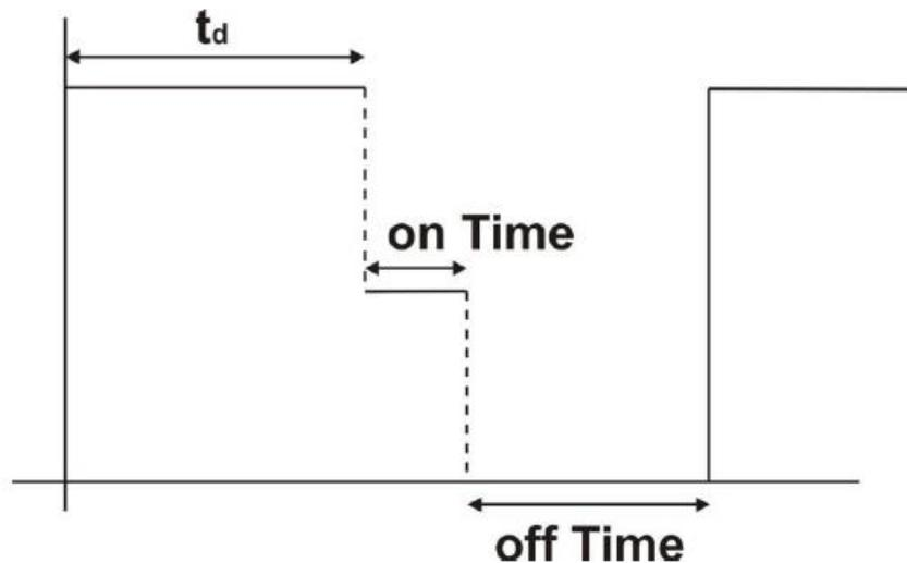
Figure 2. The three-step time intervals associated with the EDM process
