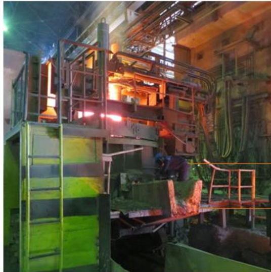
Figure 2. An arc furnace and an operator opening the tap hole
