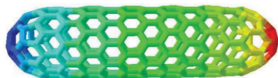
Fig. 7. Displacement contour due to an applied load to the capped tube.
