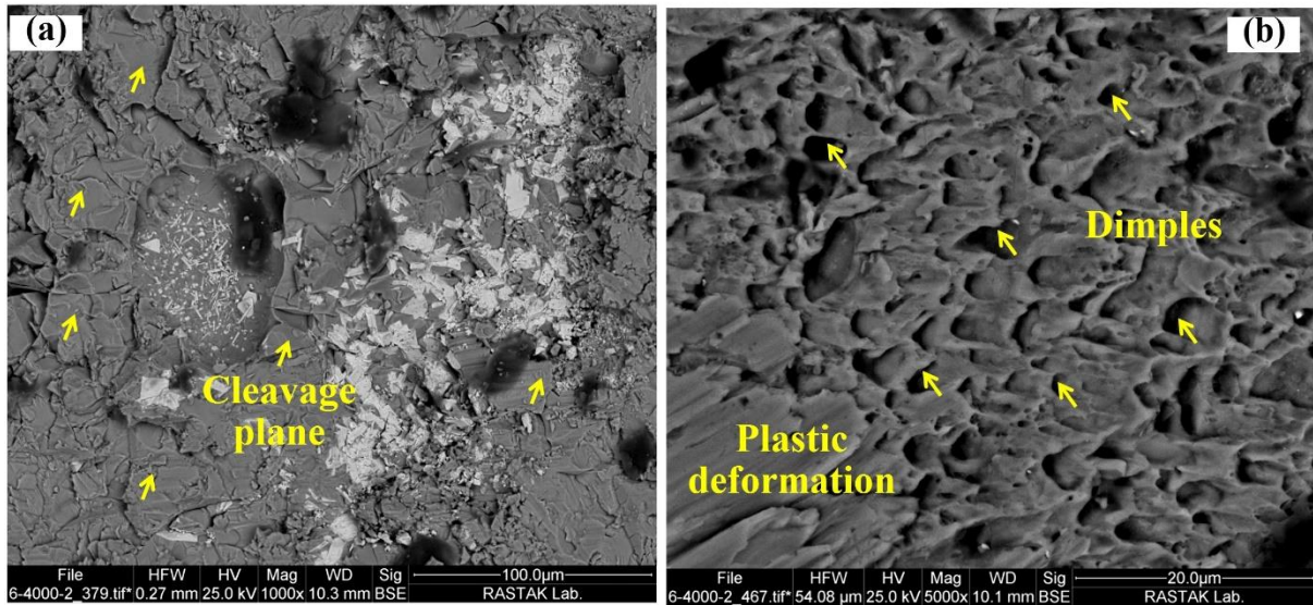
Fig. 8. SEM images of the fracture surface of the bonded sample at temperature of 1050 °C with holding time of 1 min using BNi-2 interlayer.
