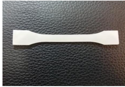
Fig. 4. The sheet in the form of dumbbells for use in the traction machine
