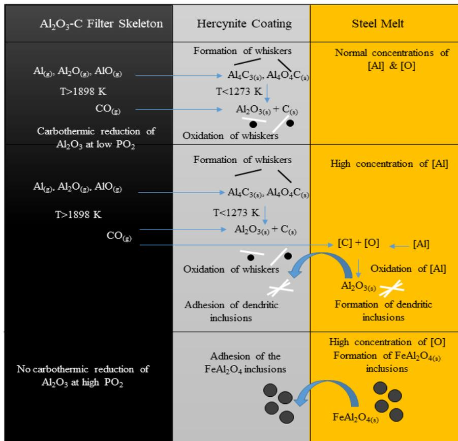
Fig. 7. Schematic illustration of the filtration phenomena of hercynite coated  $\text{Al}_2\text{O}_3\text{-C}$  filters in three different Al/Oxygen concentrations.
