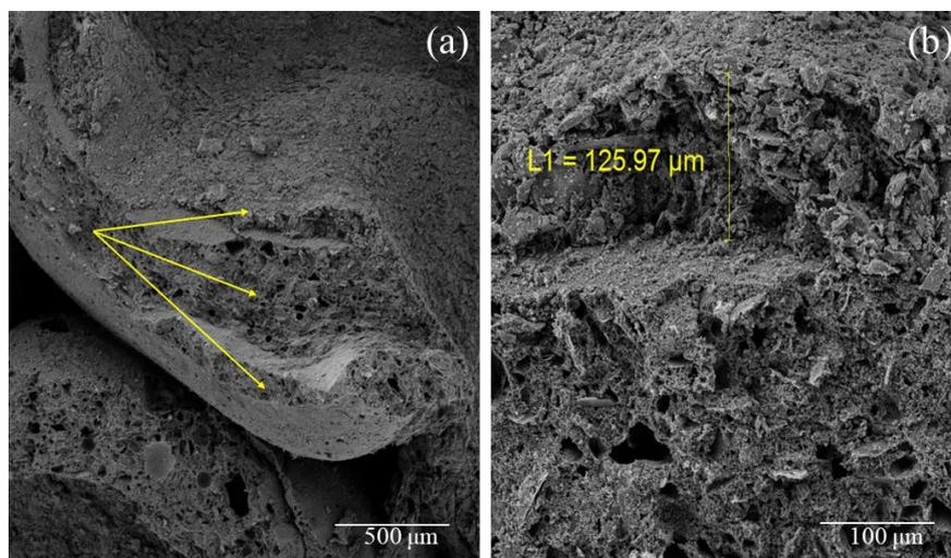
**Fig. 3.** SEM micrographs of filter surface before exposure to the steel melt; a) hercynite coating on the filter strut, b) thickness of applied hercynite coating on the filter surface.
