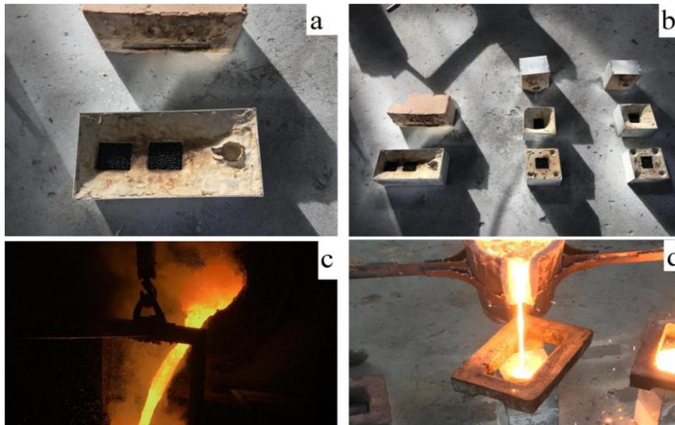
**Fig. 2.** Different stages of the molten steel impingement through  $\text{Al}_2\text{O}_3\text{-C}$  foam filters with active hercynite coating; filter preparation for the test (a and b), molten steel tapping to the main ladle with an approximate temperature of  $1650^\circ\text{C}$ ; then, transfer of the molten steel to the casting ladle with an approximate capacity of 50 kg to add aluminum as steel de-oxidizer (c), Al-killed steel casting to the molds (d).
