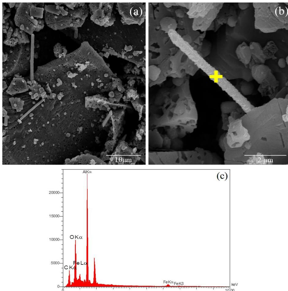
**Fig. 4.** a) and b) SEM micrographs of filter surface after exposure to the steel melt in normal oxygen activity state reveal the formation of corundum whiskers between particles of the hercynite coating; c) EDS analysis of the formed whisker marked in part b.
