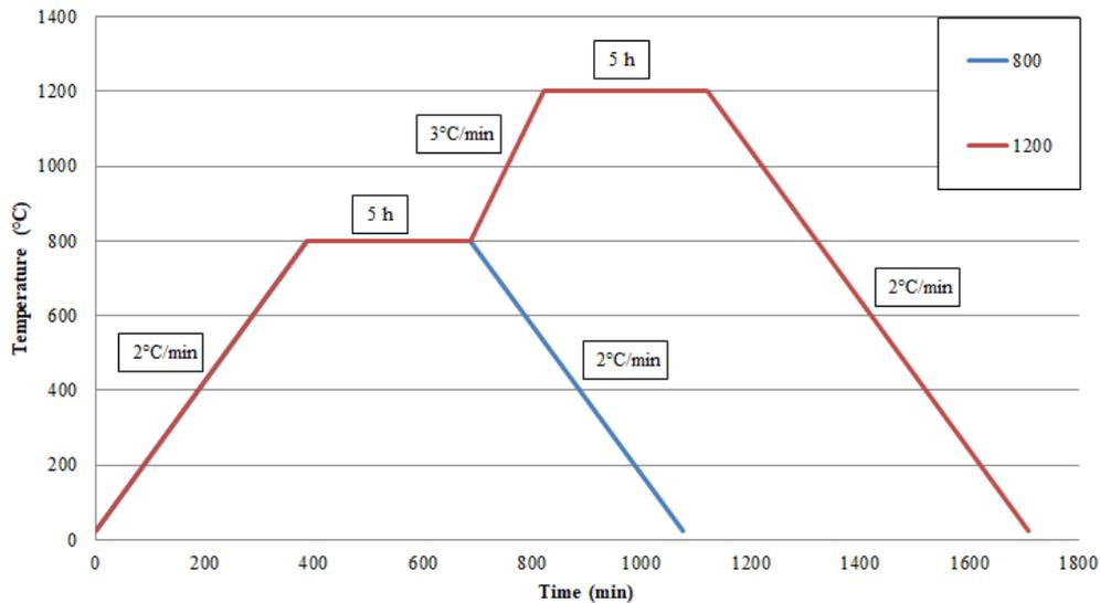
**Fig. 1.** Firing curve of Al<sub>2</sub>O<sub>3</sub>-C foam filters at 800°C and 1200°C.
