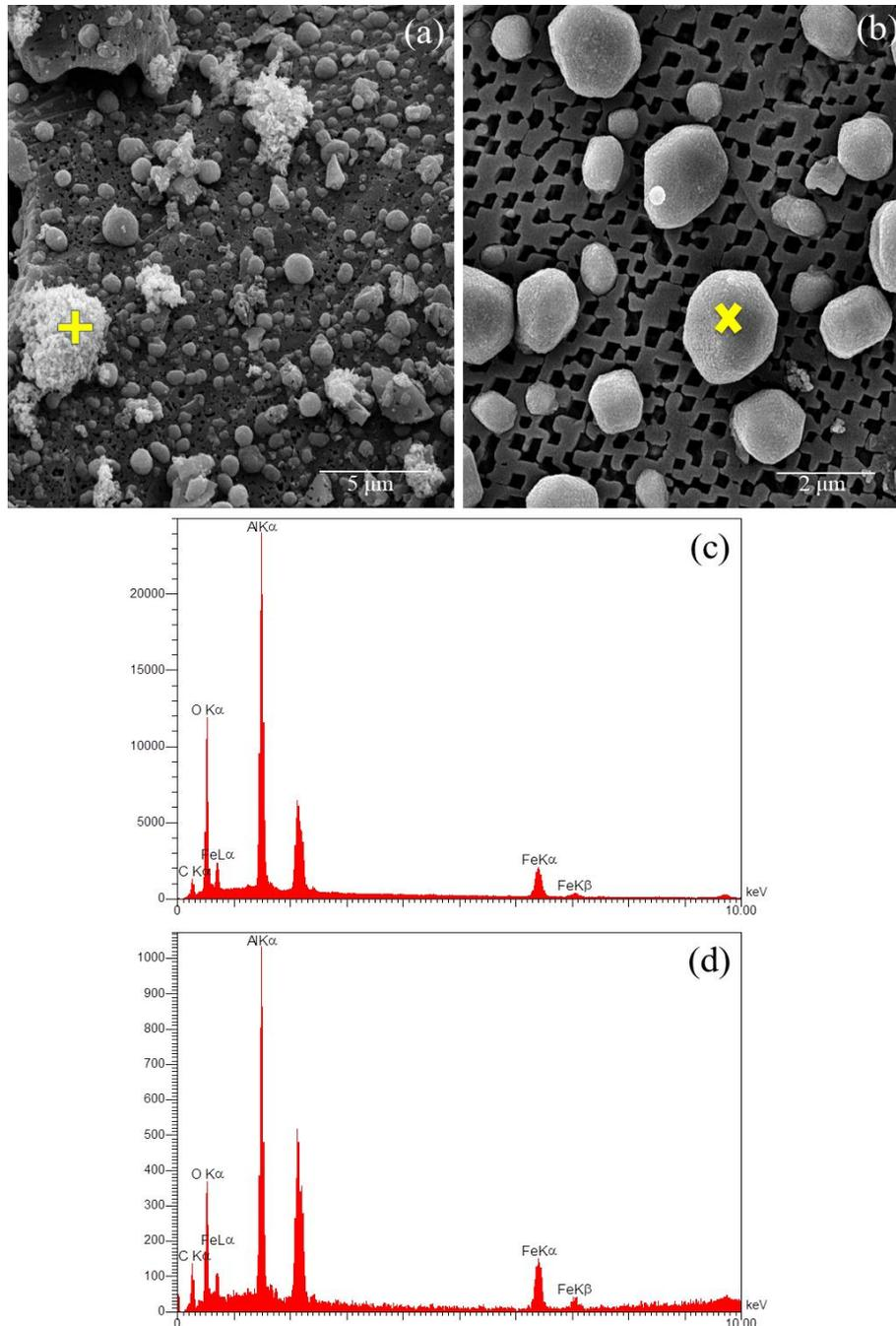
**Fig. 6.** SEM micrographs of the filter surface after exposure to the steel melt in high oxygen activity state reveal the entrapment of hercynite inclusions from the steel melt; a and b reveal different magnifications of the same concept; c and d) EDS analyses of the marked points in part a and b, respectively.
