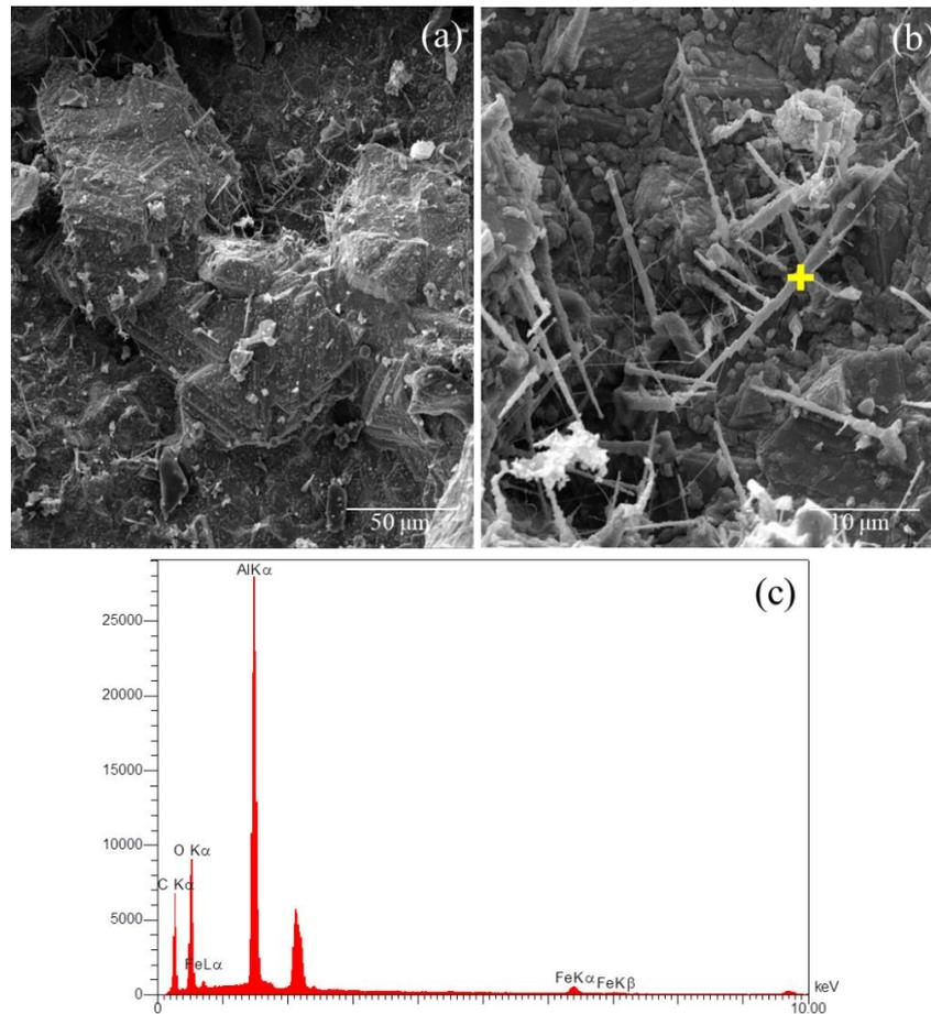
**Fig. 5.** SEM micrographs of the filter surface after exposure to the steel melt in high aluminum activity state reveal the entrapment of dendritic alumina inclusions from the steel melt as well as the formation of alumina whiskers on the surface of the filter; a) and b) reveal different magnifications of the same concept; c) EDS analysis of the formed whisker marked in part b.
