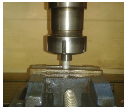
Fig. 2. Setting the electrode to electrical discharge process
