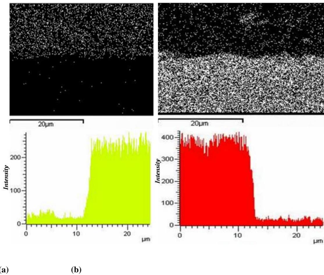
**Fig. 7.** The image of the distribution of atoms (a) Cu (b) Fe; in the form of a plate EDX at the interface of steel with bronze in a SEM microscope
