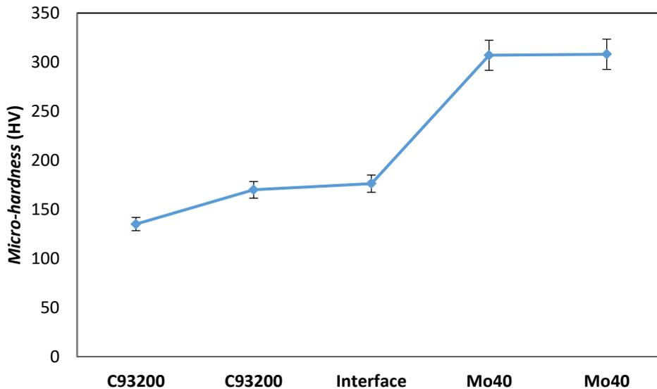
**Fig. 9.** The results of testing the micro-hardening
