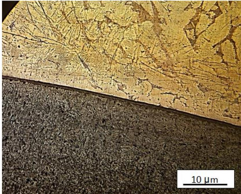
**Fig. 5.** Interface microstructure of Mo40 and C93200
