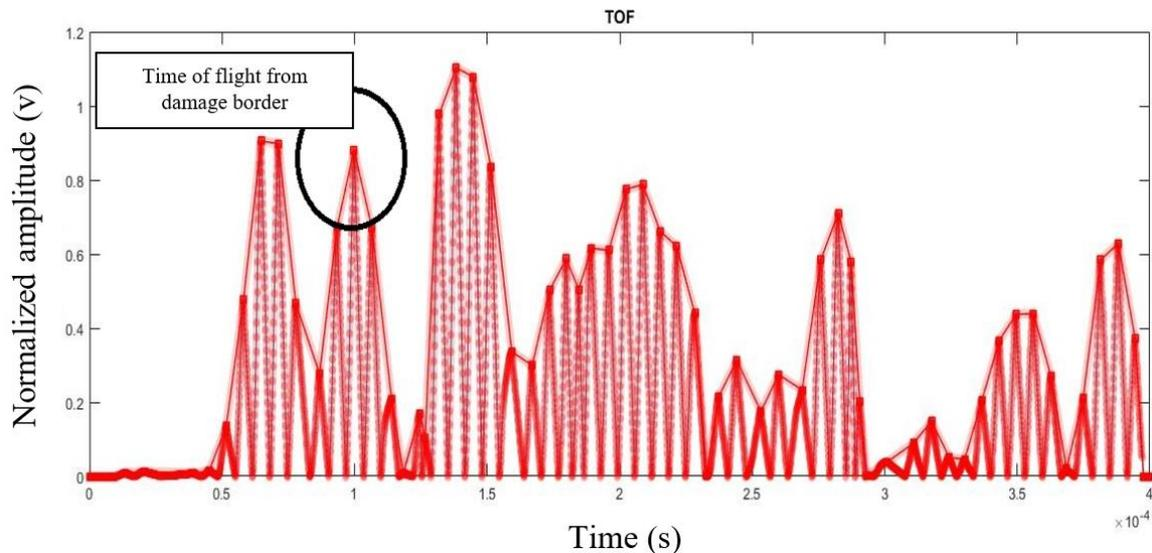
**Fig. 11.** The time of flight from the damage border.
