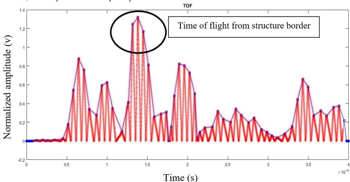
**Fig. 10.** The time of flight from the structure border.
