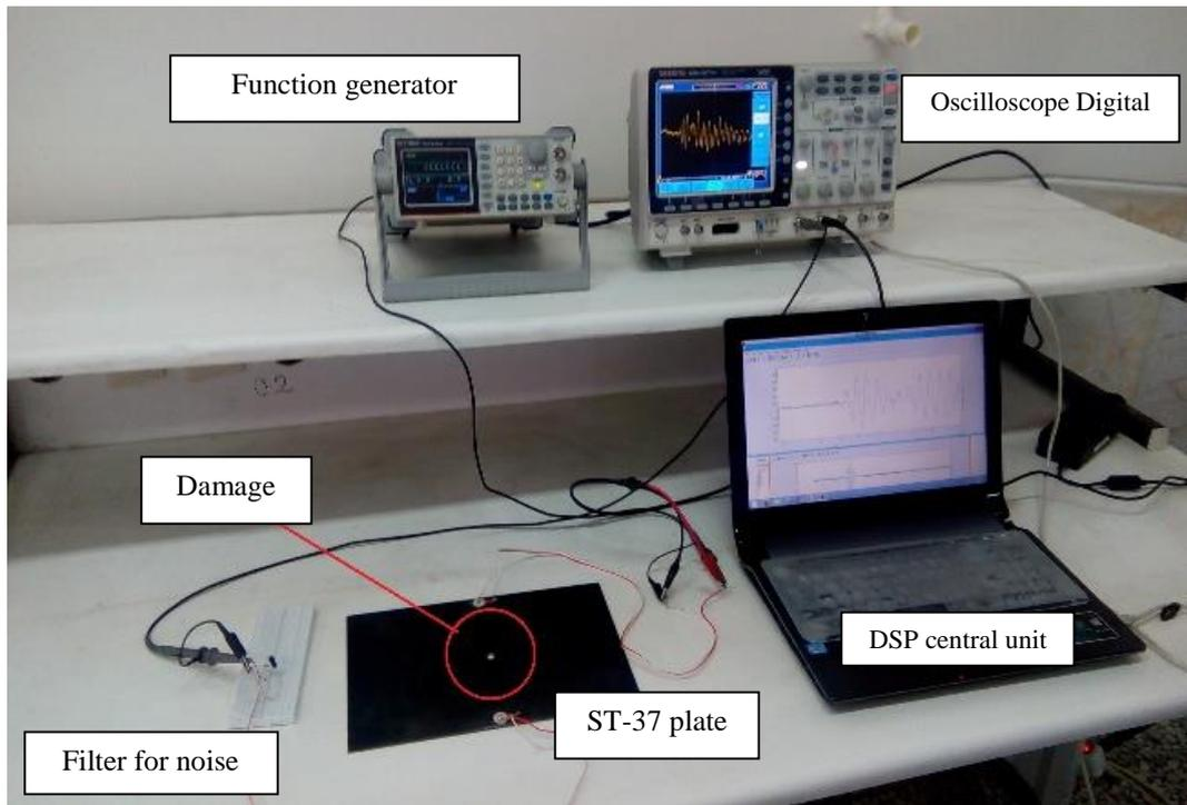
**Fig. 5.** Experimental test setup.
