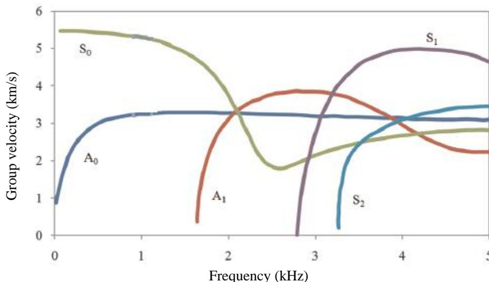
Fig. 2. Dispersion curves of the Lamb waves for steel plate [15].
