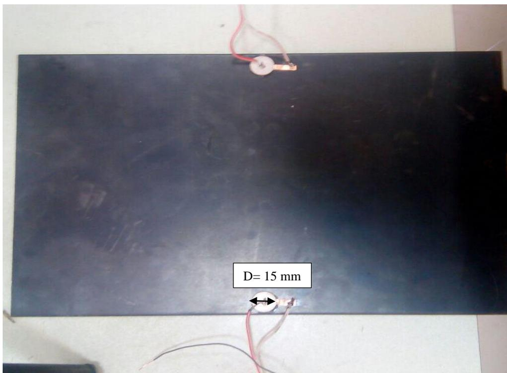
**Fig. 4.** The piezoelectric transducers attached to the steel plate.
