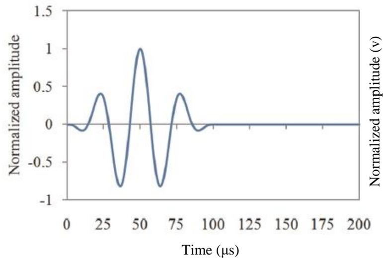
**Fig. 3.** Tune burst created by the function generator.
