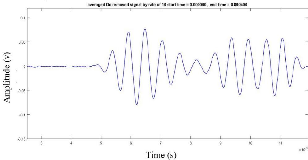
**Fig. 8.** DC noise is removed from the healthy structure signal.
