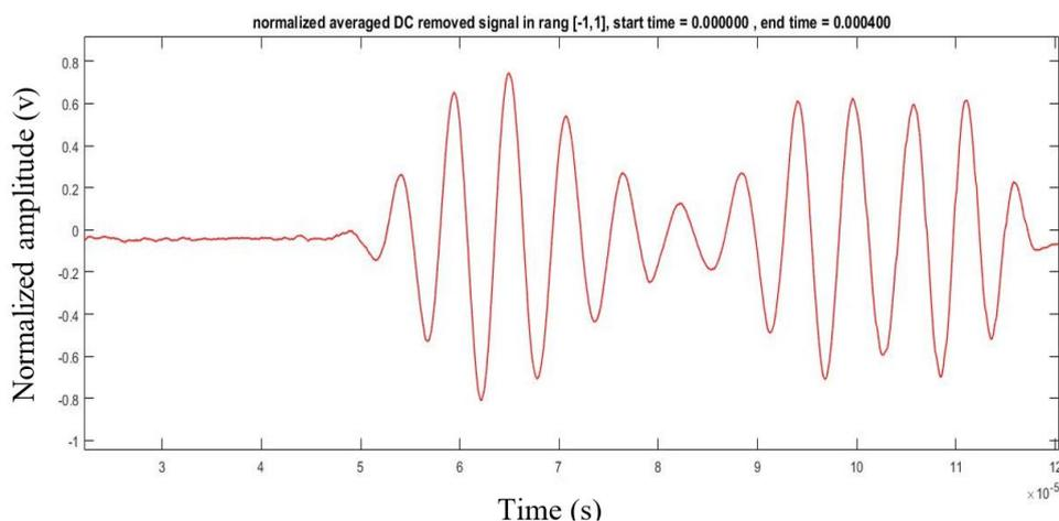
**Fig. 9.** The signals made from the damaged plate after normalizing the data.
