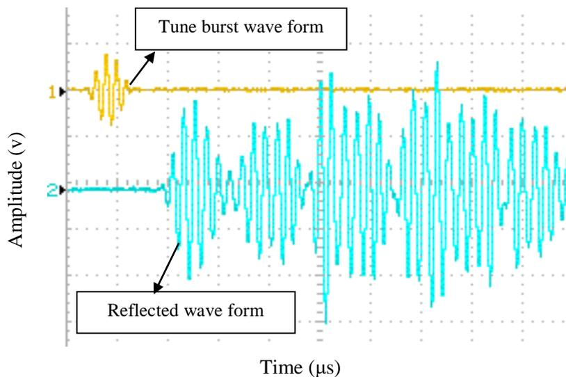
**Fig. 6.** Reflected wave from structure in oscilloscope monitor.
