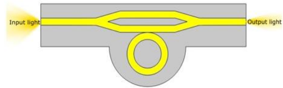
Fig. 1 Schematic of the configuration of biosensor made of plasmonic waveguide in MZI coupled to a ring resonator. The gray and yellow areas are dispersive media (silver) and sample, respectively.
