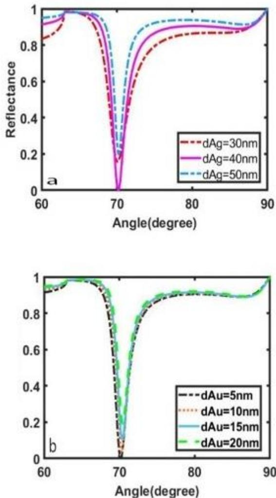
Fig. 8 The reflection spectrum of biosensor a) different thickness layer of Ag, b) different thickness layer of Au.
