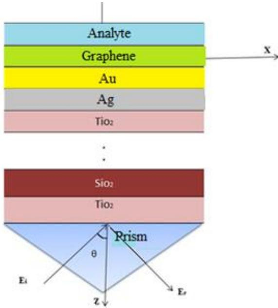
Fig. 1 Schematic view of proposed biosensor
