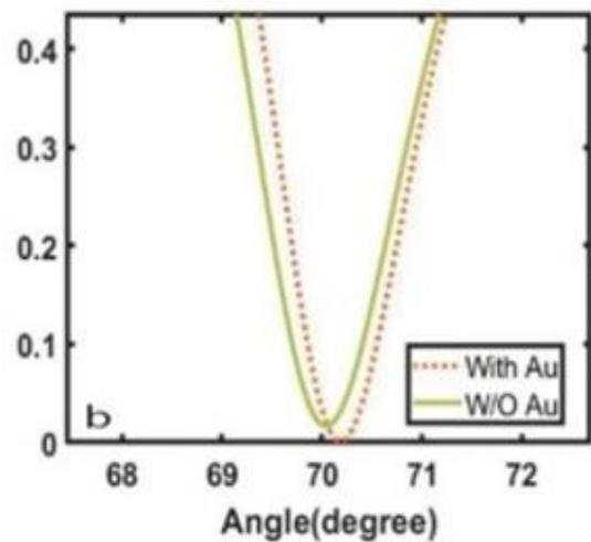
Fig. 7 a) The reflection spectrum of the biosensor with/without gold layer. b) magnification of the dip curve.
