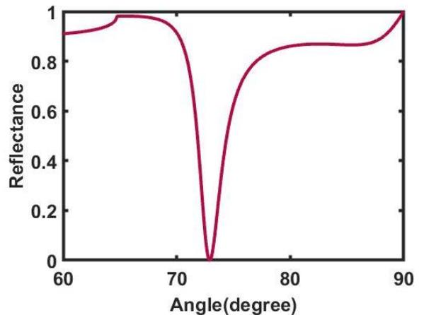
Fig. 2 The reflection spectrum of the biosensor
