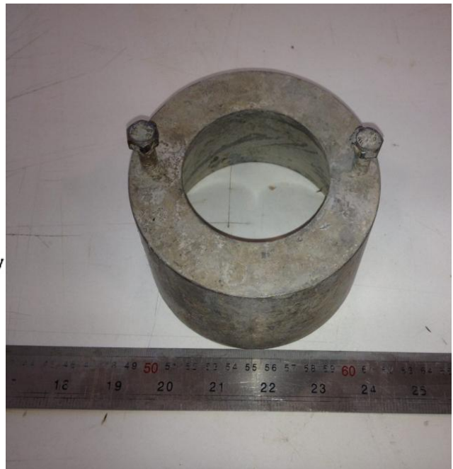
Figure 2. Configuration of mini-slump cone.
