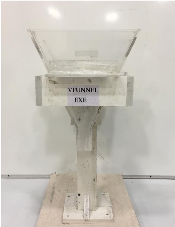
Figure 3. Configuration of mini V-funnel apparatus test.
