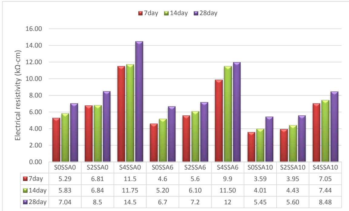
Figure 10. Electrical resistance of specimens with different ratios of waste to sand
