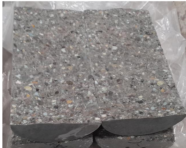
Figure 7. Control specimens after suffering one tensile loading cycle.
