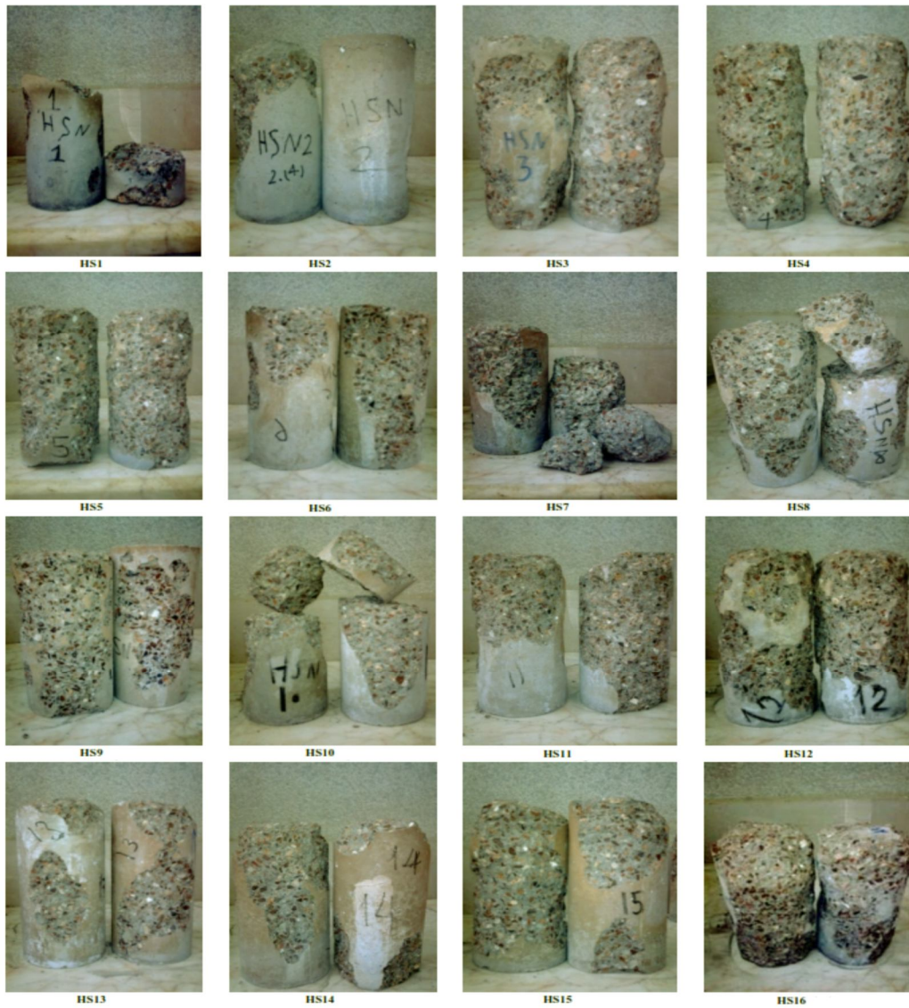
Figure 3: Schematic of concrete's samples after heating test
