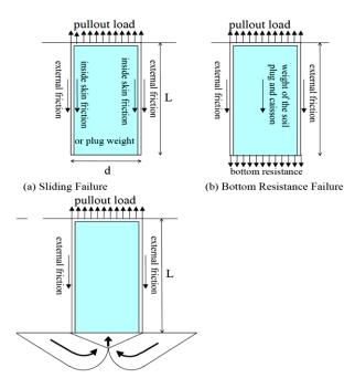
(c) Reversed Bearing Capacity Failure
