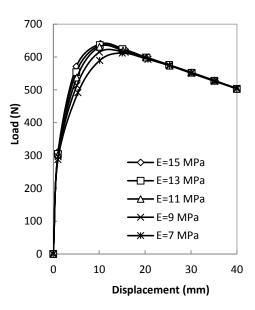
Figure 10. Yong modulus of soil on numerical pullout of suction caissons
