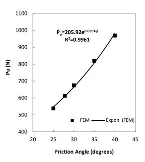
Figure 7. Soil friction angleon pull-out capacity of suction caissons
