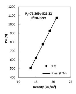
Figure 9. Pullout capacity of the suction caissons against the changes of the soil density
