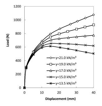
Figure 8. Soil density on pull-out capacity of suction caissons
