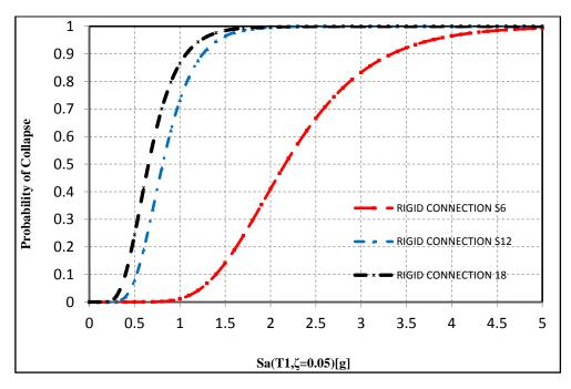
Fig 10. Collapse fragility curves of 6-, 12- and 18-stories frame considering IM=Sa ( $T_1$ ,  $\xi = 0.05$ ) and semi-rigid connections (60% rigidity percentage)
