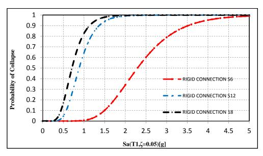
Fig 9. Collapse fragility curves of 6-, 12- and 18-stories frame considering IM=Sa ( $T_1$ ,  $\xi = 0.05$ ) and semi-rigid connections (70% rigidity percentage)
