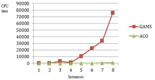
Fig. 3. Comparison of computational time between GAMS and ACO.
