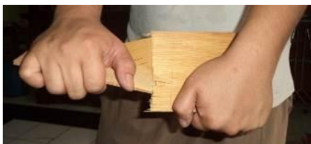
Fig. 10. The tearing method in material physical exploration
