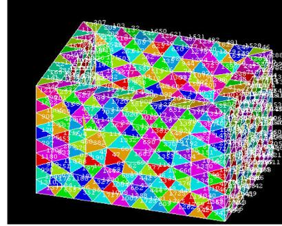
Fig. 2. FE model in ANSYS mesh with 3-D (Tetrahydal ) solid element (1737 Elements and 652 nodes)
