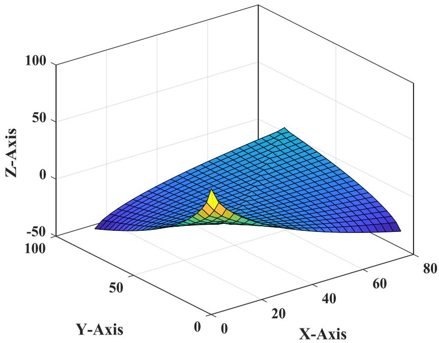
Fig. 6. The W/P deformation in fixture system subjected to clamping force=500N
