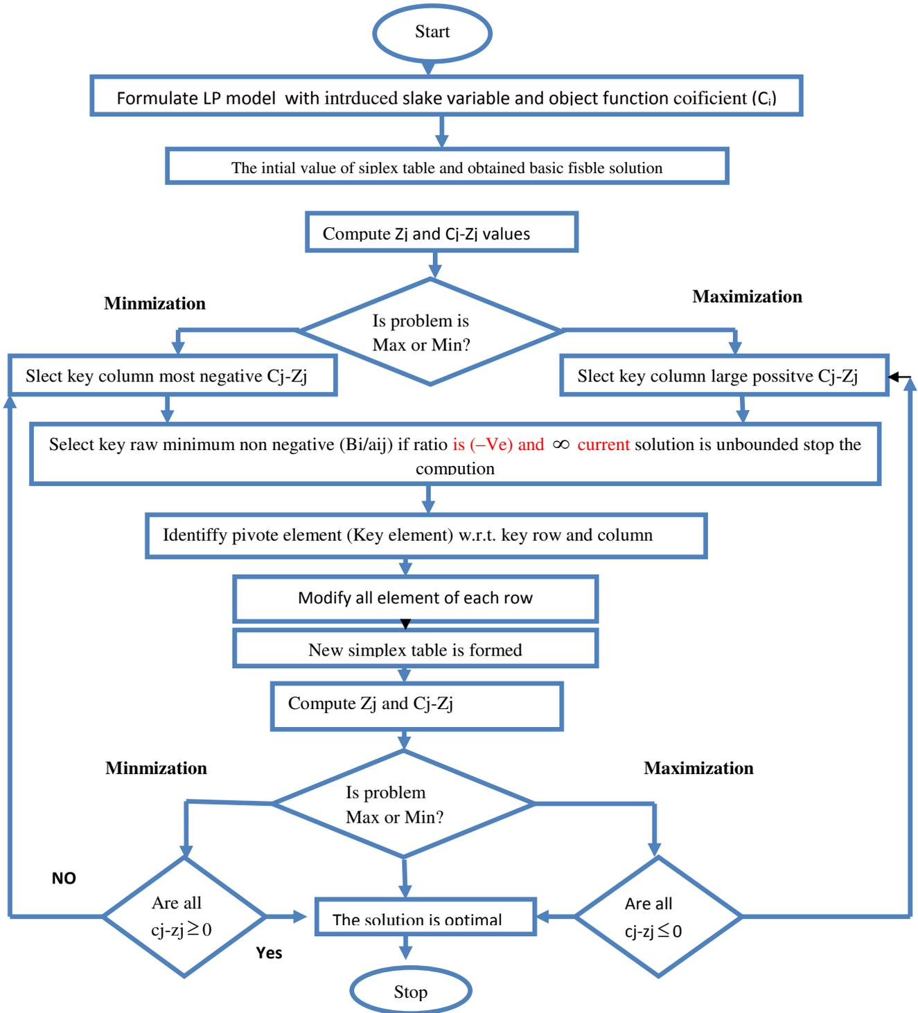
Fig. 3. The detail procedure of simplex Algorithm
