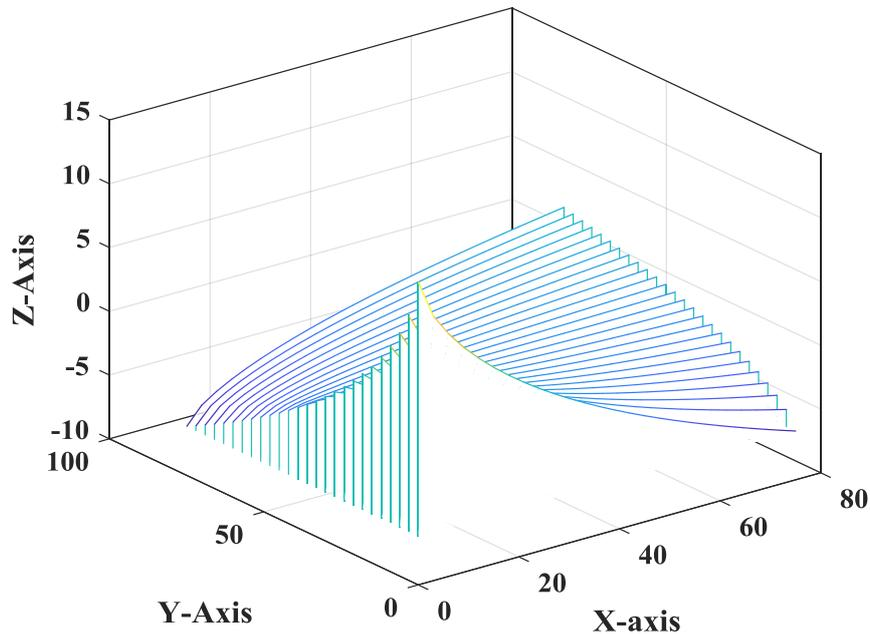
Fig.7. The W/P deformation in fixture system subjected to clamping force=100N
