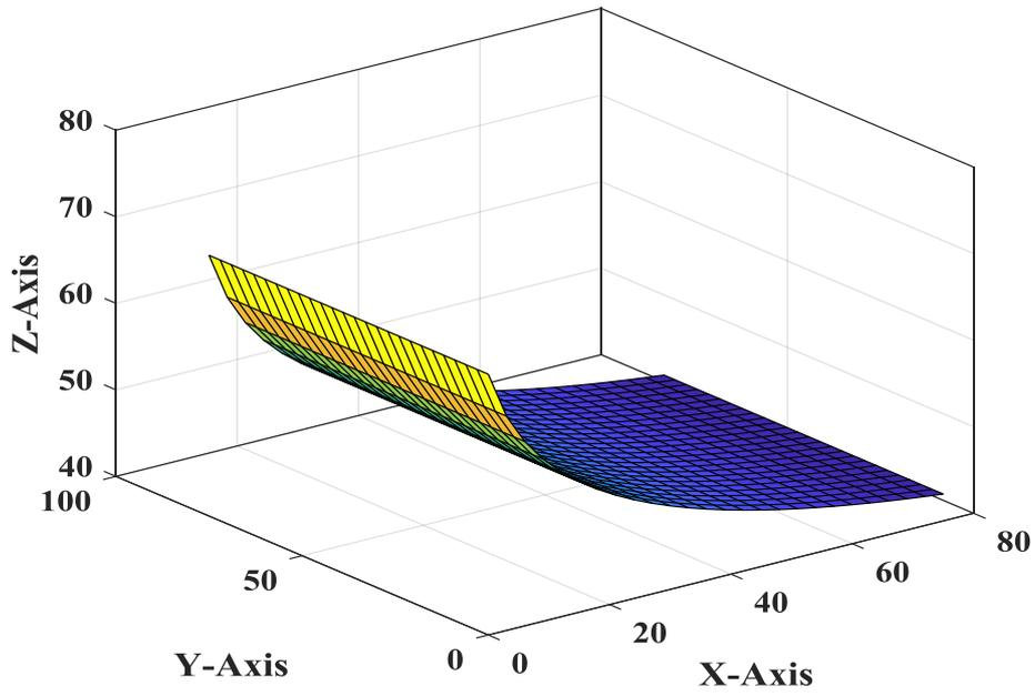
Fig.5. The W/P deformation in fixture system subjected to clamping force=100N
