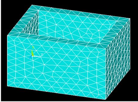
obtained unknown deformation of fixture W/P.
