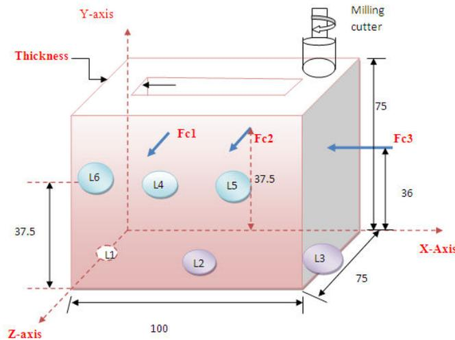
Fig.1. 3-2-1 principle W/P fixture system for End milling operation with three clamping force
