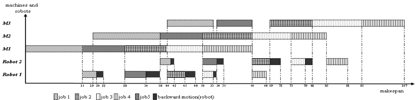
Fig. 2. Gantt chart without the effect of machine breakdown interval and robot's breakdown interval
