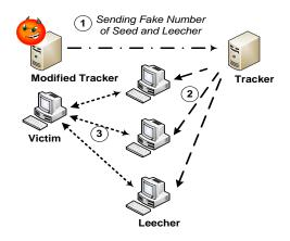
Fig. 5. DDoS attack by announcing the victim as a tracker using a Dishonest tracker.
