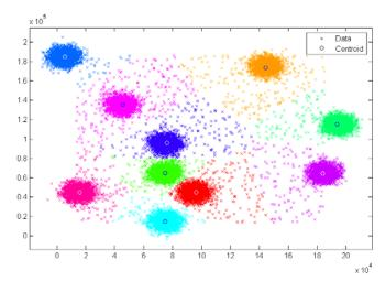
Fig. 1. Eighth iteration results of K-Means algorithm
