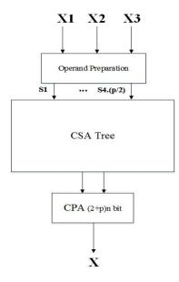
Fig. 2. Reverse Converter for proposed moduli
