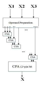
Fig. 3. Reverse Converter with CSA tree for proposed moduli
