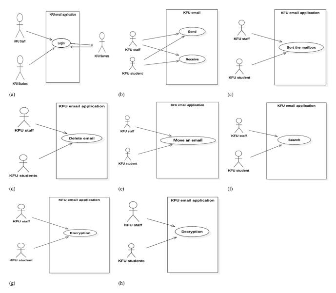
Fig. 3. The Use Case Diagrams of the functional requirements.
