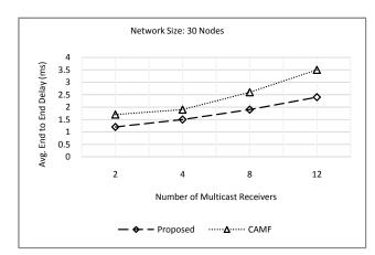
Fig. 7. Average end to end delay for a network with 30 nodes and different number of multicast receivers
