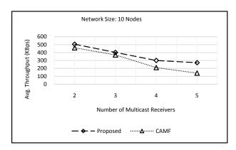
Fig. 8. Average throughput for a network with 10 nodes and different number of multicast receivers
