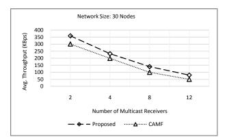
Fig. 10. Average throughput for a network with 30 nodes and different number of multicast receivers
