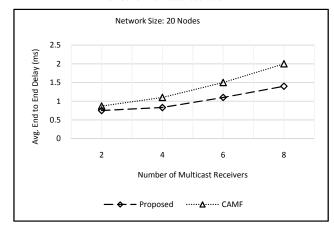
Fig. 6. Average end to end delay for a network with 20 nodes and different number of multicast receivers
