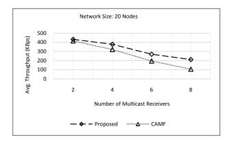
Fig. 9. Average throughput for a network with 20 nodes and different number of multicast receivers
