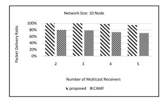
Fig. 11. Packet delivery ratio for a network with 10 nodes and different number of multicast receivers
