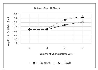
Fig. 5. Average end to end delay for a network with 10 nodes and different number of multicast receivers
