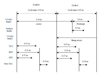
Fig. 14. Timing of instruction fetch stage.
