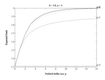
Fig. 5. Self-Aligned expected instruction fetch with prefetching (n=4).
