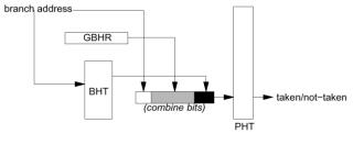
Fig. 9. Alloyed branch prediction.
