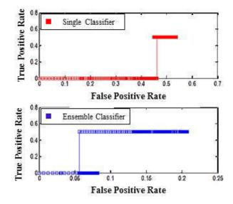
Fig. 12. *ROC* curve of the proposed system (blue) against the singleclassifier case (red). The proposed method attains a shorter threshold value to coordinate (0,1).
