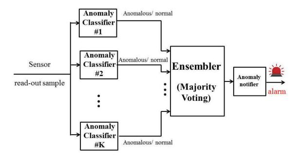
Fig. 4. The process of diagnosis and notification of anomalies in the proposed system based on majority voting.
