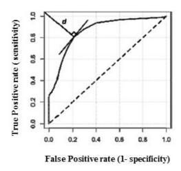
Fig. 6. The "ROC" curve and the optimum threshold value concerning the sensitivity and specificity [10].
