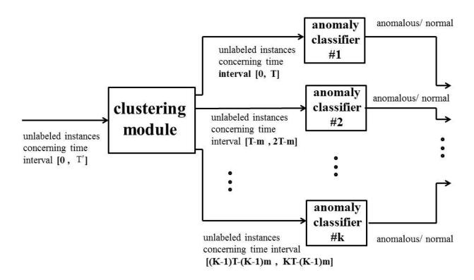
Fig. 3. Creation of K classifiers in the proposed method: The interval [0, T'] is divided into K sliding windows, each of which with length *T*. In each step, the window *T* is sliding *m* points. So, every window will have overlap with size *m* with its previous and next windows.
