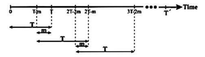
Fig. 2. Sliding window scheme in the proposed method: Each interval T contains tagged read-out samples of WSN sensors. Each window has m-size overlaps with its previous and next windows.
