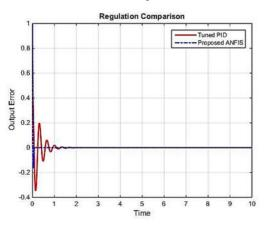
Fig. 11. comparison between PID optimized controller and suggested optimized controller in regulation state
