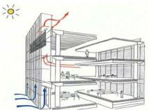
Fig. 1. One type of double skin facade function (http://cajaislant.com/blog-cajaislant/, 2018)
