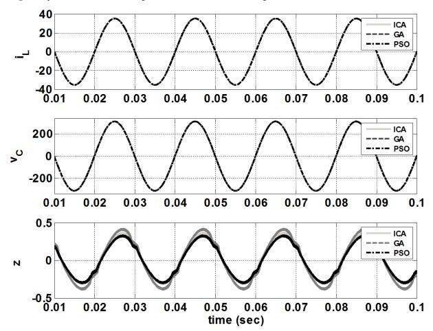
Fig.5. Simulation results of the grid-connected inverter during steady-state operation
