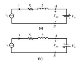
Fig.2. Equivalent circuit of grid-connected inverter in switching mode a) u = 1 and b) u = 0
