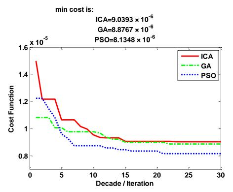
Fig.4. Objective function convergence in ICA, GA and PSO algorithms
