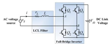
Fig.1. Power topology of the grid-connected inverter
