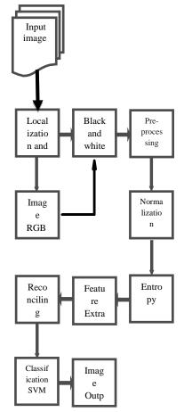
**Fig .2.**Block diagram of the proposed face recognition system in this paper
