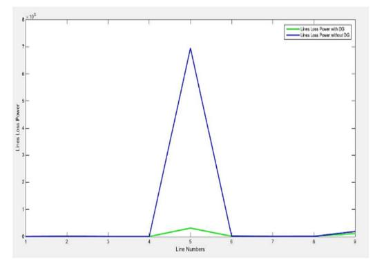
Fig.4. Line losses comparison before and after DG installation in 10-bus network
