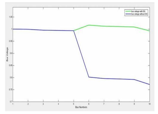
Fig .3. Voltage profile comparison before and after DG installation in 10-bus network
