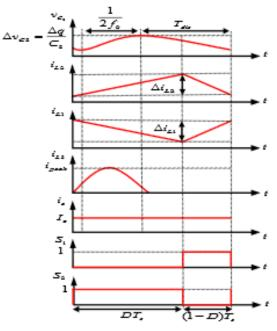
Fig.5. Waveforms for selecting the reactive element
