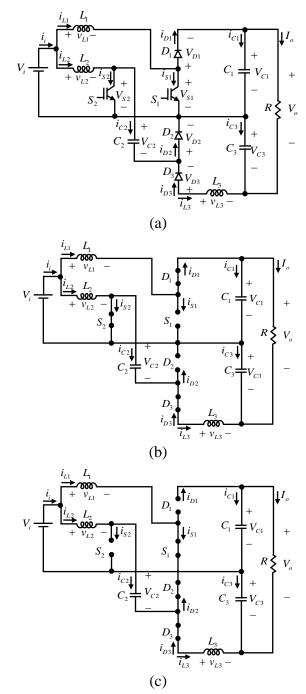
**Fig.1.** (a) the converter circuit provided; (b) the equivalent circuit of the converter in the time interval  $DT_s$ ; (c) the equivalent circuit of the converter provided in the time interval  $(1-D)T_s$
