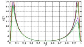
**Fig .3.** The voltage gain versus to the working cycle with the ESR of inductors
