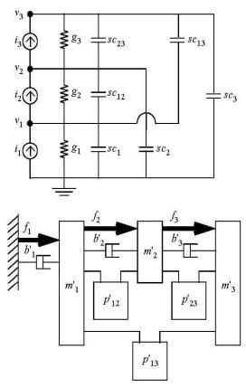
Figure.14: Model of a 3-DOF serial robot.
