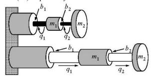
Figure.8: Redundant rotary & prismatic actuators.
