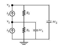
Figure.9: System models of redundant actuators
