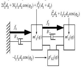
Figure.12: Mechanical model of a 2-DOF serial robot.
