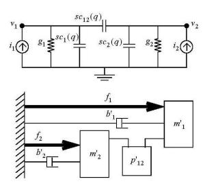
Figure.13: Model of a 2-DOF parallel robot.
