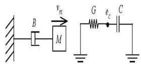
Figure. 2: LC circuit and mechanical equivalent.
