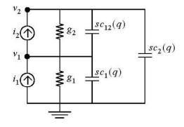
Figure.11: Electrical model of 2-DOF serial robot.
