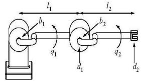
Figure.10: 2-DOF serial robot.
