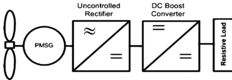
**Fig.2.** a brief block diagram of the proposed PMSG wind-energy system [2].
