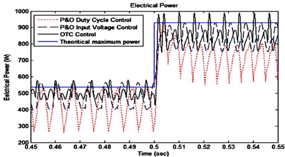
**Fig.14.** the output power response produced by the pmsg generator [2].
