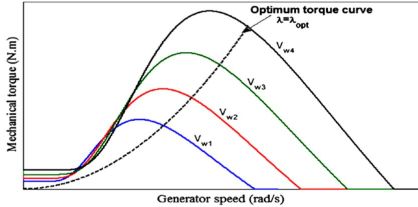
**Fig.7.** the torque-speed characteristic curve for a series of wind speeds.
