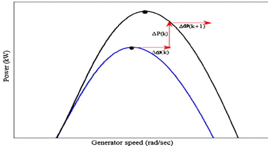
**Fig.11.** the HCS control losing its track ability under changing wind conditions and traveling downhill instead of the uphill climb [24].
