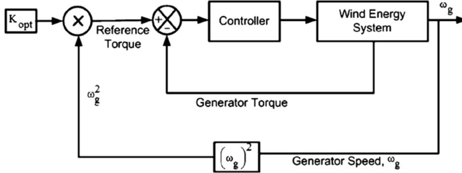
Fig.6. the block diagram of optimal torque control mppt method [2].
