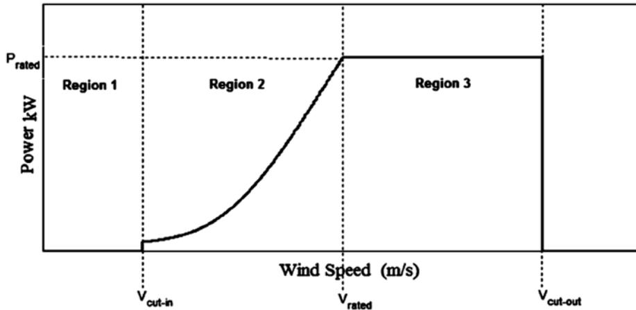
**Fig.1.** Ideal power curve of a wind turbine
