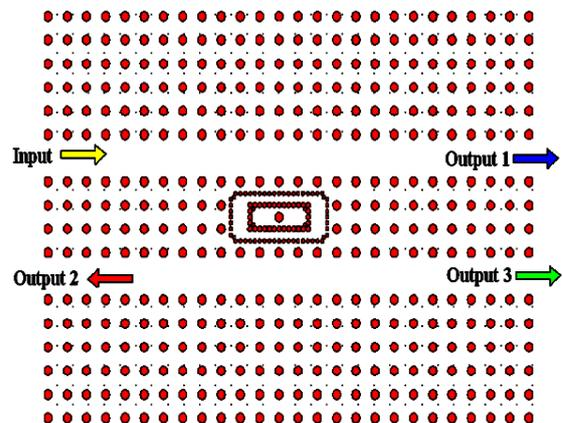
Fig.3. Schematic of structure of removed and added filter based on photonic crystal nested rectangular resonator
