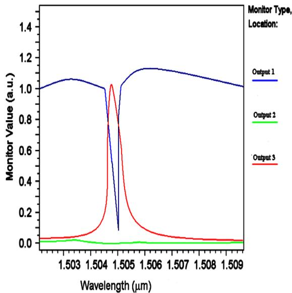
**Fig.4.** Normalized transmission spectrum of removed and added filter based on a photonic crystal rectangular resonator with a wavelength of 1550 nm
