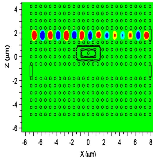
**Fig.6.** Electromagnetic field intensity for frequency of 1330 nm
