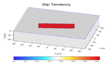
**Fig.3.** The calculated slip tendency of Tabriz fault
