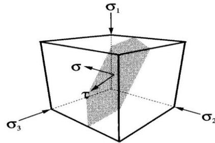
**Fig.1.** The normal stress  $\sigma_n$ , and shear stress  $\tau$ , on a desired level of tension in the field defined by the main compressive stresses  $\sigma_1$ ,  $\sigma_2$ ,  $\sigma_3$
